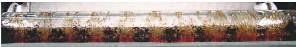
FIGURE 24. Segregation of two types of particles in water. The filling level F = 0.357 . The concentrations of the black silicon particles and brown resin particles are 4% and 16%, respectively. The rotational speed is 306 r.p.m.
