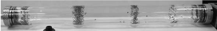
FIGURE 16. Band formation of particles due to capillarity. The liquid is glycerine with a density of 1.173 \text{ g cm}^{-3} , and the particles are polymer particles with a density of 1.034 \text{ g cm}^{-3} and a diameter of 0.65 \text{ mm} . The filling level F is 0.105 and the particle concentration is 4.8\% . The rotational speed \Omega = 5.45 \text{ r.p.m.} , \beta = 1.443 , average film thickness D_a = 0.753 \text{ mm} , minimum film thickness D_{min} = 0.605 \text{ mm} , D_{min}/d_p = 0.931 . Band formation 15 h after the beginning of rotation is shown in the figure.
